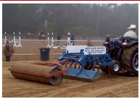
The Water Roller tube is 20" in diameter with 1/4 wall thickness
